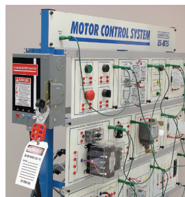
Grounded Panels with lockout / tagout
