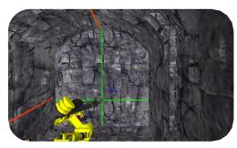
Drilling single stope holes using a single boom, grade and laser lines
